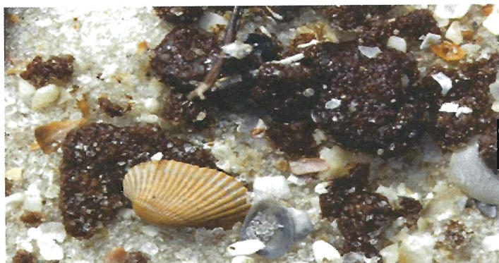
MC252 Oil Characteristics: Brown color, shiny or dull surface, mixed with sand and shell
